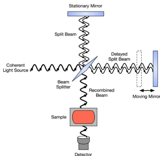
Fig. 2: FTIR Michelson interferometer
